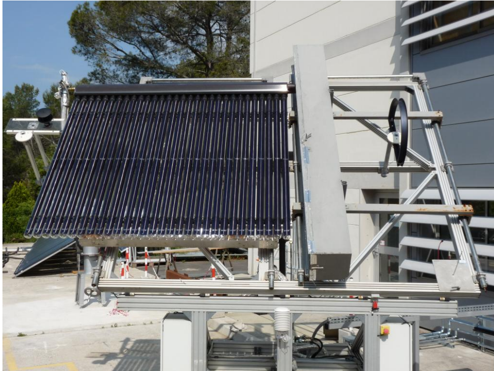
Figure 5: test with an automatic tilt (normal incidence is verified by the gnomon on the bottom right)
